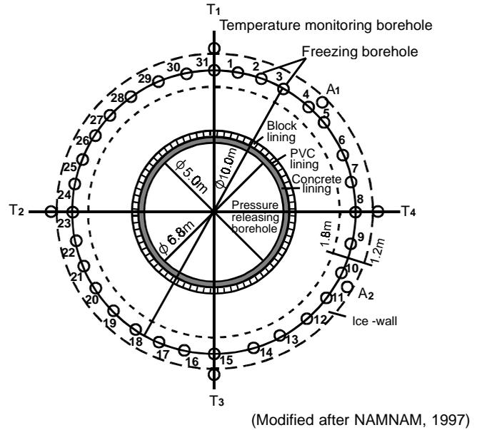
Fig 3. Arrangement of freezing borehole for cage shaft sinking.
