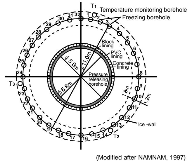
Fig 4. Arrangement of freezing borehole for skip shaft sinking.
