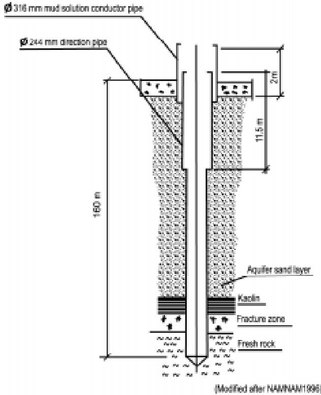
Fig 2. Longitudinal section of freezing borehole in MHMP.
