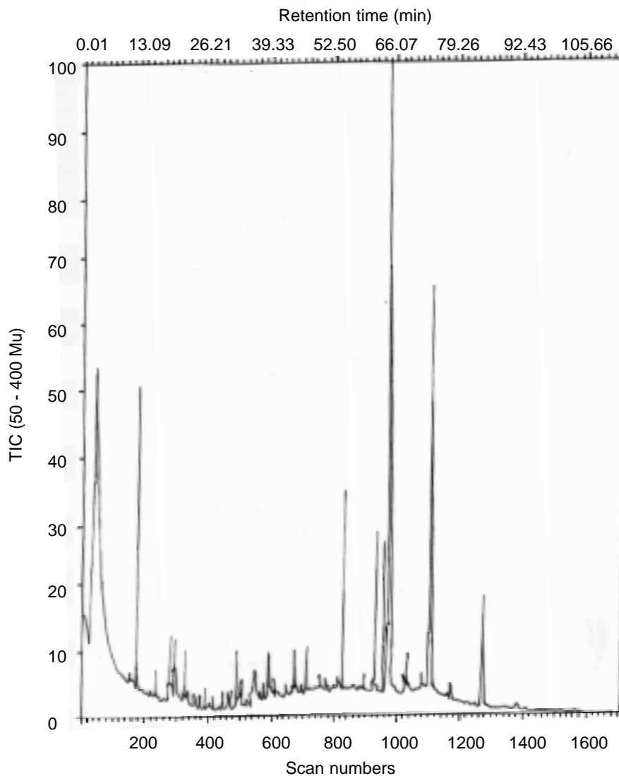
**Fig 3.** Total ion current chromatogram of methyl esters of fatty acids HMWCFE of fraction II.
