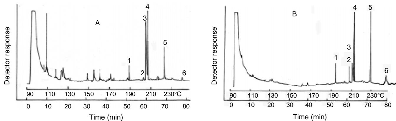
**Fig 1a & 1b.** GLC separation of methyl esters of *C. lindemuthianum* (A) Partially purified HMWCFE fraction I, (B) HMWCFE fraction II, oven temperature was increased from 90°C to 230° at 2°/min, peak numbers correspond to the methylester listed in Tables 1 and 2.
