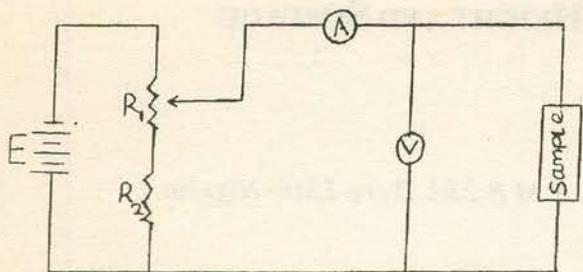
**Fig 1.** Circuit diagram for current (I) - voltage (V) measurements sample - Enclosed in a crocheted maintained at room temperature. V - Voltmeter (Volts), A -Ammeter (MA),  $R_1$  - Fixed Resistor,  $R_2$  - variable Resistor, E-Source of power.
