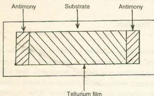
**Fig 2a.** Final configuration of the deposited samples.
