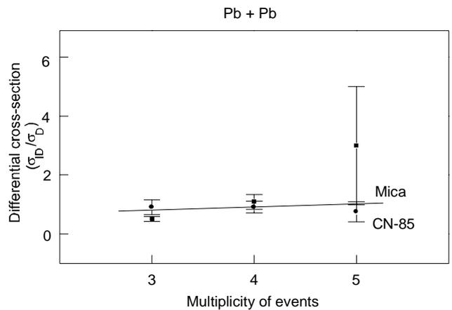
**Fig. 4.** Differential cross-sections of indirect to direct events for each multiplicity shown for both the reaction and both types of detectors. Error bars are the statistical errors.
