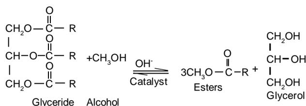
Fig. 2. Transesterification reaction for biodiesel production.
