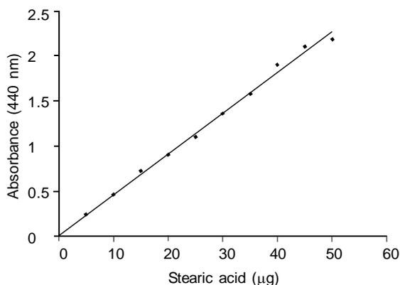
Fig. 1. Standard curve for free fatty acid determination.
