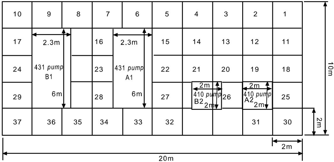
Power of motors: A<sub>1</sub> = 200 KW; A<sub>2</sub> = 75 KW; B<sub>1</sub> = 55 KW; B<sub>2</sub> = 230 KW
