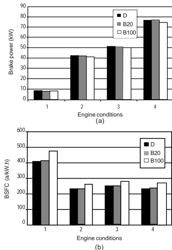
**Fig. 2.** Effect of biodiesel on (a) brake power and (b) BSFC, at different conditions.
