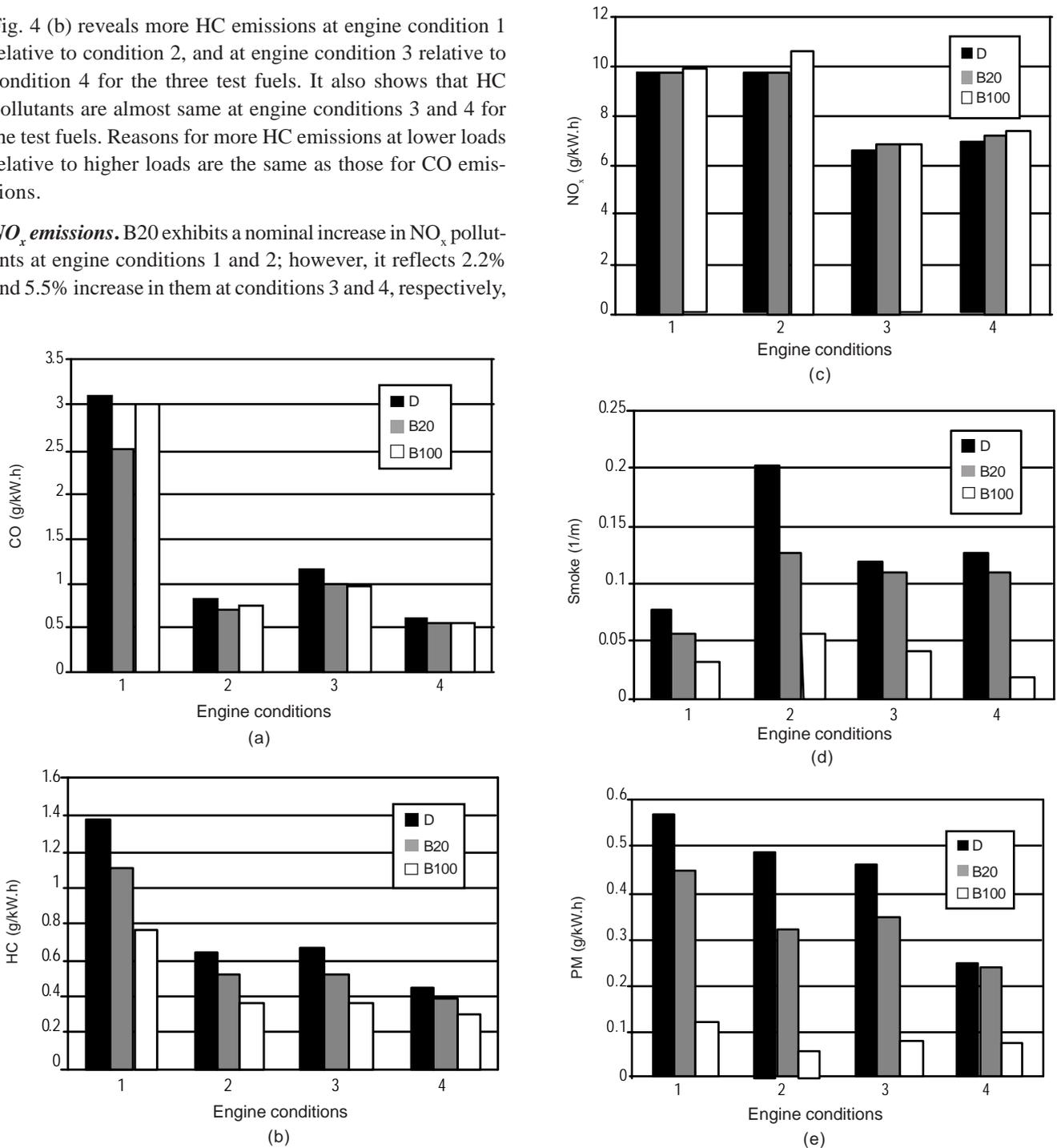
**Fig. 4.** Effect of biodiesel on (a) CO; (b) HC; (c) NO<sub>x</sub>; (d) smoke and (e) PM emissions.
