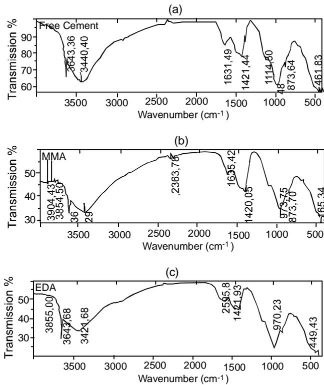
**Fig. 5.** Infrared spectra of 28 days-hydrated sample: (a) blank cement; (b) with methylmethacrylate additive; (c) with ethylenediamine additive.
