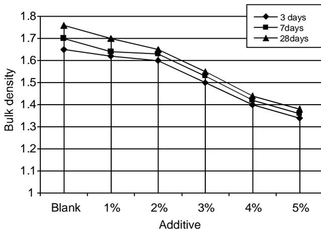
Fig. 1. Effect of methylmethacrylate on bulk density of high strength portland cement.
