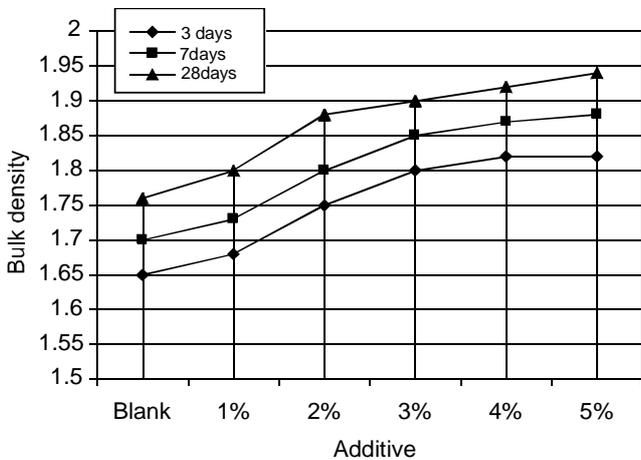
Fig. 2. Effect of ethylenediamine on bulk density of high strength portland cement.
