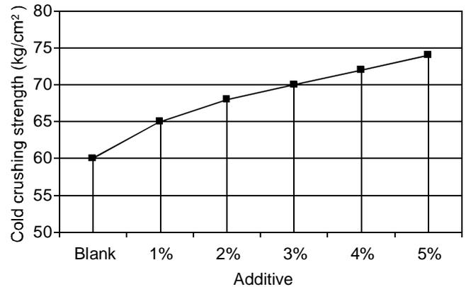
Fig. 4. Cold crushing strength of 28 days-hydrated cement with ethylenediamine.
