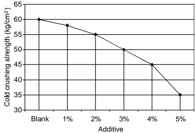
Fig. 3. Cold crushing strength of 28 days hydrated cement with methylmethacrylate.
